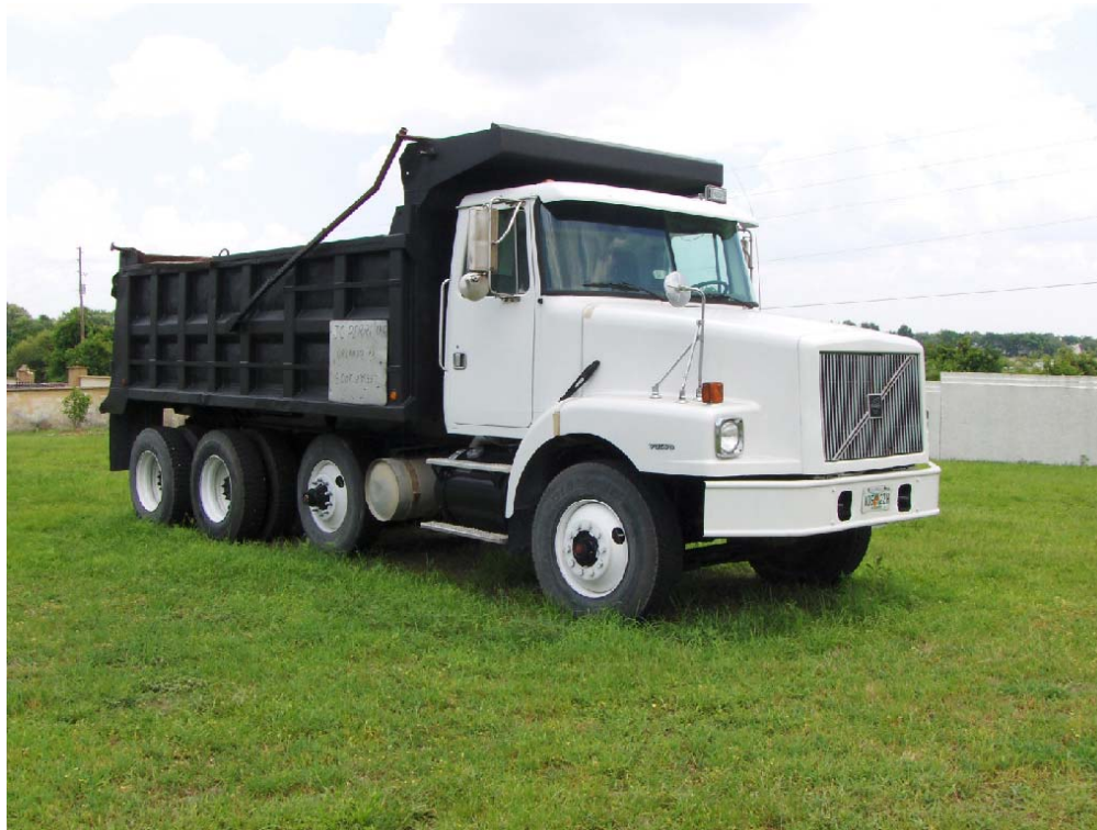
18 Cubic Yard Dump Truck
